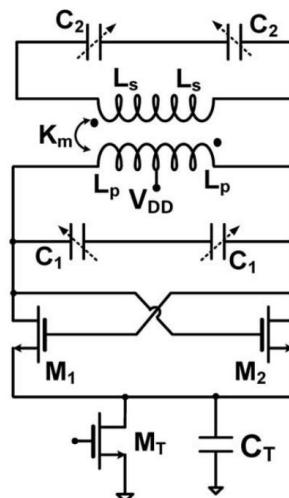
Figure 1: Schematic of a class-F oscillator [1].
